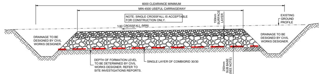
SECTION THROUGH NEW SITE ROAD CONSTRUCTION PHASE (CBR BETWEEN 2% and 4%)
